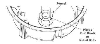
Flip **Hopper Top** upside-down and mate to **Hopper Bottom**.
