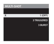
**3 TRIGGERED** - Up to three photos are captured per event with an approximate one second delay between each capture. Each subsequent photo after the first requires an individual trigger. This allows for multiple potential image captures of the same event while reducing the chance of empty images if the subject moves out of the field of view after the first shot.
